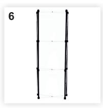
6. Continue, in the same way, attaching all the metal bars in a vertical line until you get four vertical lines of three bars each: two lines in the front and two lines in the sideback. Now the PopUp frame (C) is assembled.
